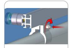
Using hex key turn bolt clockwise to tighten tube clamps, securing graphic header to backwall.
