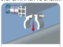
Once graphic is attached to stand-offs and extrusion, position tube clamps (TC-30) onto backwall.
