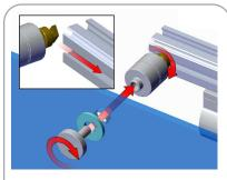
Attach graphic to stand-offs and extrusion with washer & other end of stand-off. Turn clockwise to secure.
