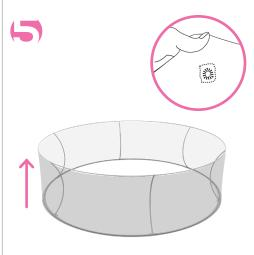
Place the graphic underneath the frame. Pull up the graphic and cover the entire frame. Make sure the printed graphic faces outwards and the prehemmed holes are aligned with the top screws. Insert the eyehooks along the pre-hemmed holes.
