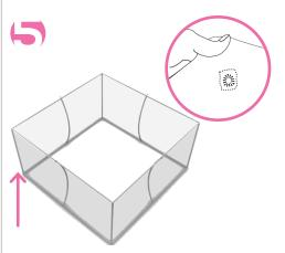
Place the graphic underneath the frame. Pull up the graphic and cover the entire frame. Make sure the printed graphic faces outwards and the prehemmed holes are aligned with the top screws. Insert the eyehooks along the pre-hemmed holes.
