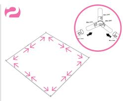
Connect the bottom straight horizontal tubes (Blue Colored Label: B) and corner connectors. Snap them together.
