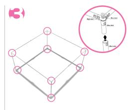
• Then connect the vertical straight tubes (Blue Colored Label: T & B) to the top and bottom corner connectors.
