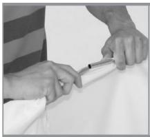
4. When the required amount of fiberglass poles (A) are inserted, secure the end fiberglass poles (A) together. Relieving pressure makes this easier, so ask a second person to push gently on the fiberglass pole (A) section directly across from the section to be connected. Repeat 1-4 for bottom pole sleeve.
